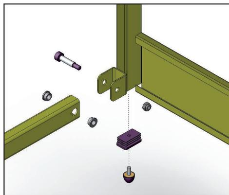
Screw the rubber stops -Nb 8- in the perforated plastic foot -Nb 6- and fix them in the panel tubes - Nb 1- Insert the plastic caps 50 x 30 -Nb 7- on the top of the panel tubes -Nb 1- Fix the beams
