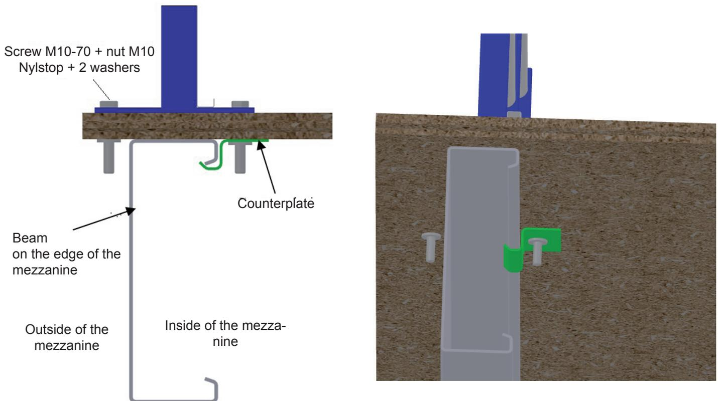
Fix the uprights onto the flooring using 2 screws M10, 70mm long, class 8.8, and 2 nuts M10 Nylstop, 2x2 washers and the counterplate.
