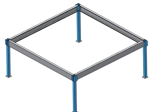
**Fix the non-load-bearing beams** to close the module
