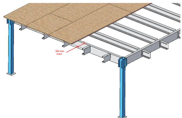
Semi-beams in the non-load-bearing direction
