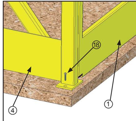
Fix the whole elements to the floor using screws H M 10 x 70 -Nb 19- and self drilling screws diam. 5 x 40 -Nb 18- The main wedges of the ground - Nb 4- will have to be reinforced under the floor (one simple layer of 38 mm or a double layer of 22 mm) with a counter wedge of 3 mm -Nb 5-
