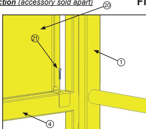
Position the side protection of the safety gate rep. 20 on the ground rep 4. Fix it with the 4 self drilling screws rep 21 on the ground rep 4.
