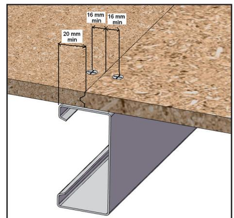
The self-tapping screws must be positioned at least 16 mm from the effective edges of the panel (See drawing opposite). The screw head must sit flush with the upper surface of the flooring.
