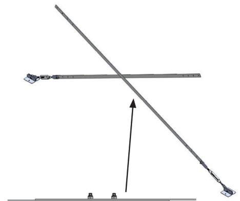
The cross-bracing rod (ID 2), the tensioner (ID 3) and the tensioner supports (ID 1) are fixed using the screws and nuts HM12 with a lockwasher (ID 4 and 5). The entire set is fixed to the floor, at the foot of the mezzanine upright, using the ground anchor bolts (ID 6) while observing the rules defined on page 10, and, at the top of the upright, on the upright connector using screw and nut HM12 with a lockwasher (ID 4 and 5).
