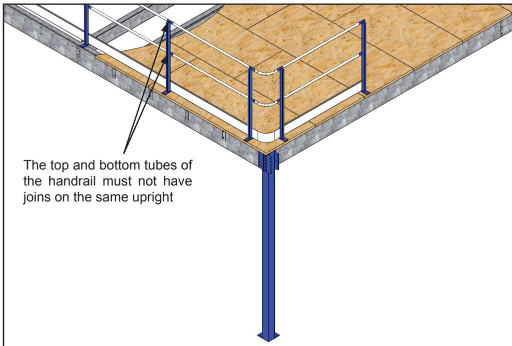
Position the handrails and fix them in place using the self-tapping screws (D4.2mm, L19mm) provided
