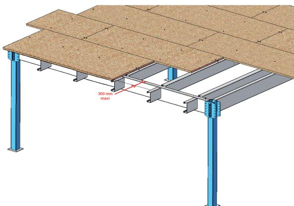
Semi-beams in the load-bearing direction
