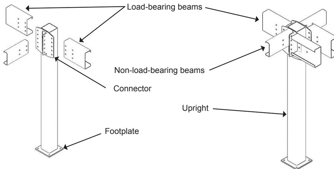
We distinguish between load-bearing beams, which receive joists, and non-load-bearing beams. Non-load-bearing beams are mounted parallel to the joists.
