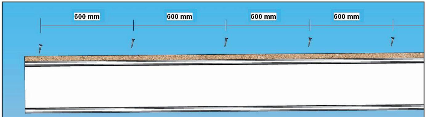
The panels must be laid in a «brick wall» arrangement, taking care to ensure that:
