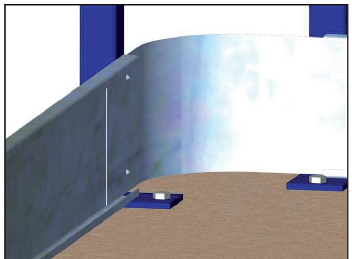
Position the plinths and fix them in place using the self-tapping screws (D4.2mm, L19mm) provided
