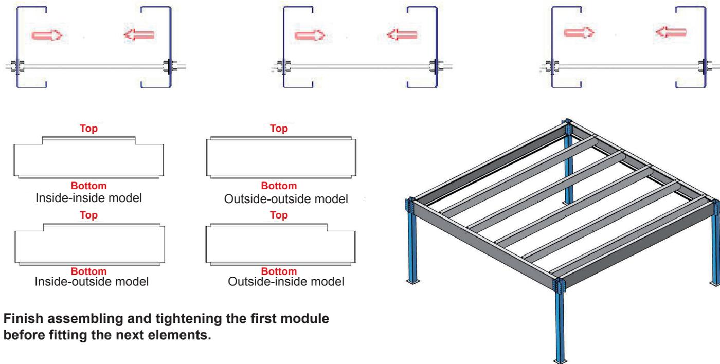
**Finish assembling and tightening the first module before fitting the next elements.**
