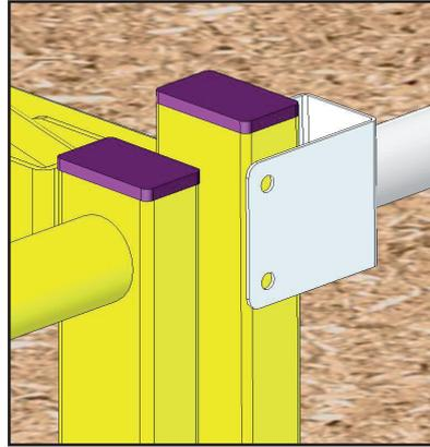
Align the safety gate to the handrail, as close as possible to border the mezzanine, respecting the capacity limit of the floor.
